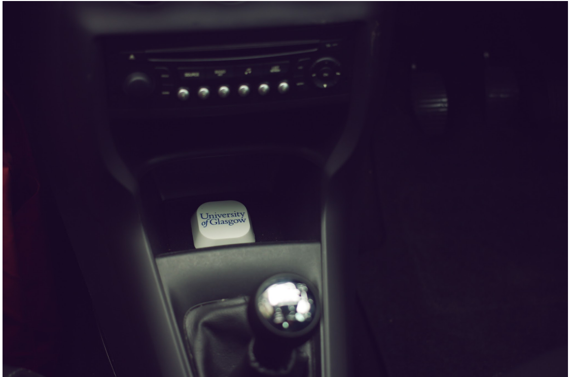
Figure 6.8: Kontakt.io Low Energy Bluetooth (LE) beacon placed in a car.
