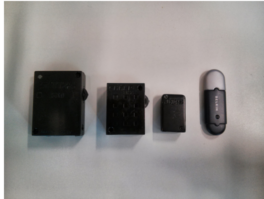
Figure 5.16: SHAKE SK6, SHAKE SK7, JAKE and USB Bluetooth beacons.
