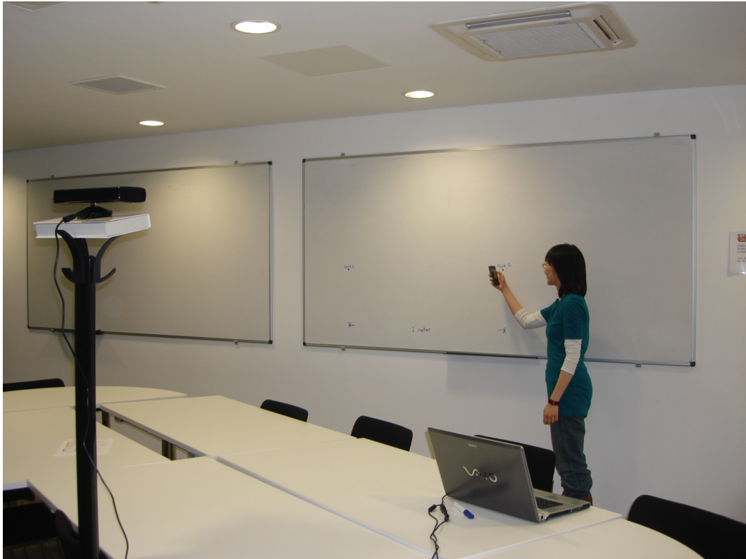
Figure 4.3: Experiment setup. The participant is pointing the mobile device in front of Point 1 in the forward facing condition and is being tracked by the Kinect.
