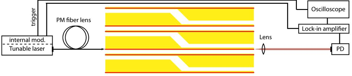
**Figure 5.4:** Schematic of the transmission loss measurement setup.
